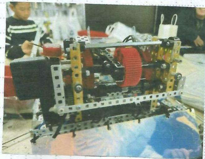
We also made the adjustments according to the previous solution to solve the problem in the ports. However, we found that the position of the pressure gauge also effects the configuration, resulting in inconsistent landing points. So we change the position of it.
