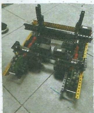
Additionally, we try to change the screws to nylon screws to reduce the weight. However, it need repeatedly using a lighter to secure the screws and nuts, which can be too cumbersome. Besides, the center of gravity would be raised, increasing the likelihood of Robot tipping over.
